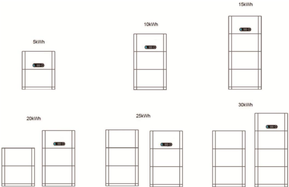
Figure 2.3-1 Storage Capacity Description
